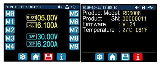
You can press '**SHIFT' + 'MENU'** to enter the system setting menu, and then press the right button three times to enter the system information menu as shown above. You can view the SN number, firmware version and system temperature here.
